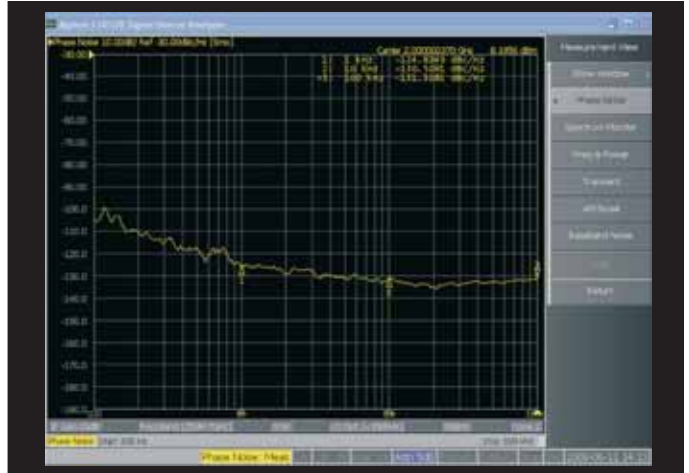
Figure 56 · QuickSyn phase noise at 2 GHz output.
